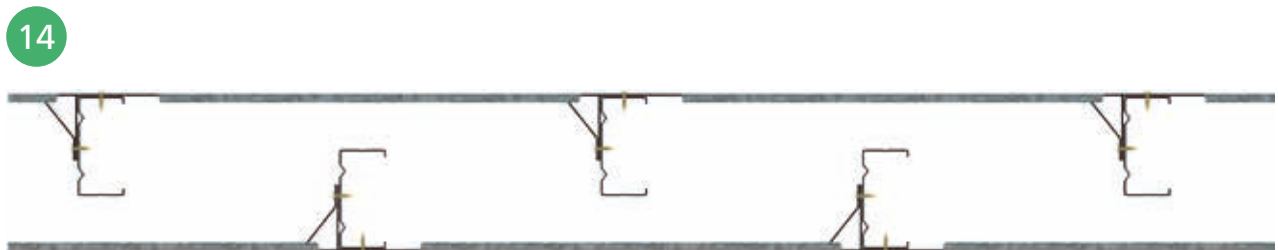
■ PLAN VIEW OF STAGGERED STUD FRAMING WITH FAST-FIX NOGGING INSTALLED BOTH SIDES
