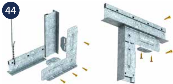
The XD10 securely joins two tier grid components at a 90° angle. Bend down tabs secure the Clip to the grid. Screws provide a structural connection.
