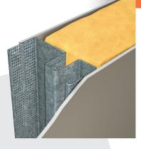
Noise is actually vibration. A normal stud conducts the vibration across its web, and sound is transmitted via anything that reacts to it by vibrating. The Rondo QUIET STUD® is overall bigger in surface area than a standard wall stud. Therefore, the sound (vibration) has further to travel and tends to weaken in intensity across the wall, resulting in a more acoustic efficient wall system.
