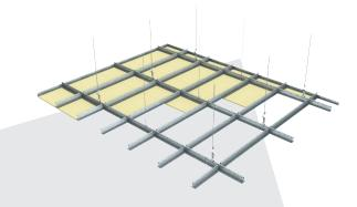
The Rondo Xpress® Drywall Grid Ceiling System is light-weight and simple to install.
